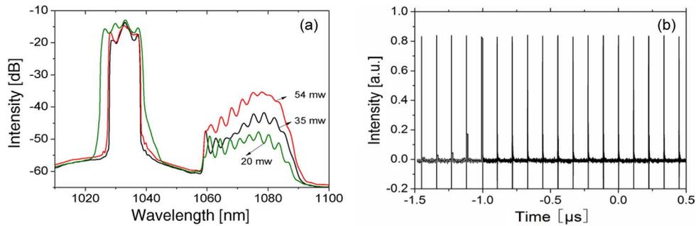
Fig. 2. (a) 1032-nm output spectra of the mode-locked fiber laser at different output power (20 mW, 35 mW, 54 mW). (b) Output pulse trains of 1032-nm mode-locked laser.
