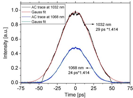
Fig. 4. Autocorrelation trace of the mode-locked laser at 1032 nm and 1068 nm.
